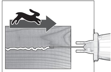
To avoid potential damage of the tool, always allow motor to come to a complete stop before using the orbital action selector.
